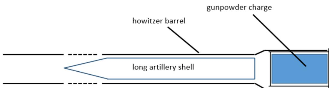
A projectile with a protective layer is not limited to a smooth barrel. A rifled barrel can also be used. Long length provides a large internal volume and stable flight aerodynamics. In practice, it turns out a planning ammunition with a high initial speed, which does not require an aircraft to launch. The technical wear of the barrel also has little effect.
